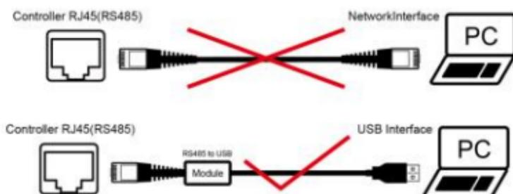
**WARNING:** Connecting the controller with PC network communication port by network cable is forbidden. It may cause the damage to the components of the controller.
